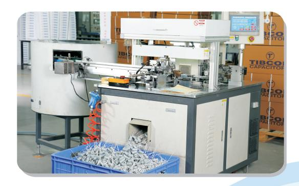
Precise pressure & temperature control to minimize damage to the Capacitor during the process. Since manual systems are subjected to pressure & temperature variations.
